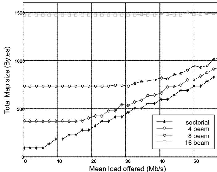
FIGURE 7. Simulation results of the minimization strategy: total map size for a 4-, 8- and 16-beam positions SBA
