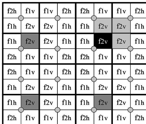
FIGURE 2. Considered reuse pattern: two frequencies and two polarisations. The grey coloured act as co-channel interference sources. The dark grey sectors are the dominant co-channel interferers.
