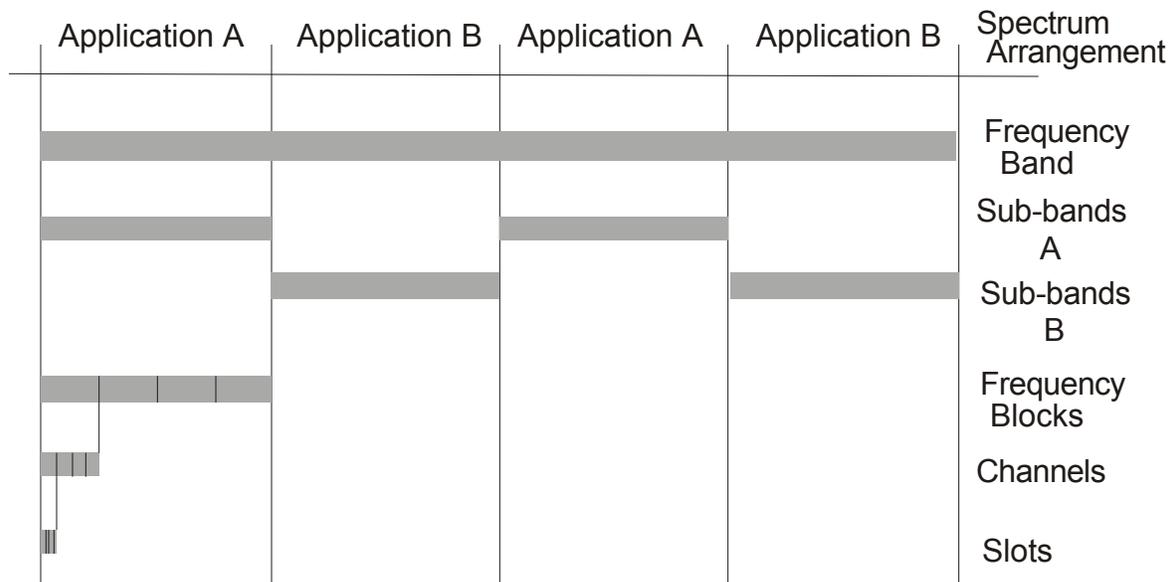
NOTE: Guardbands can occur at any frequency edge in this diagram
