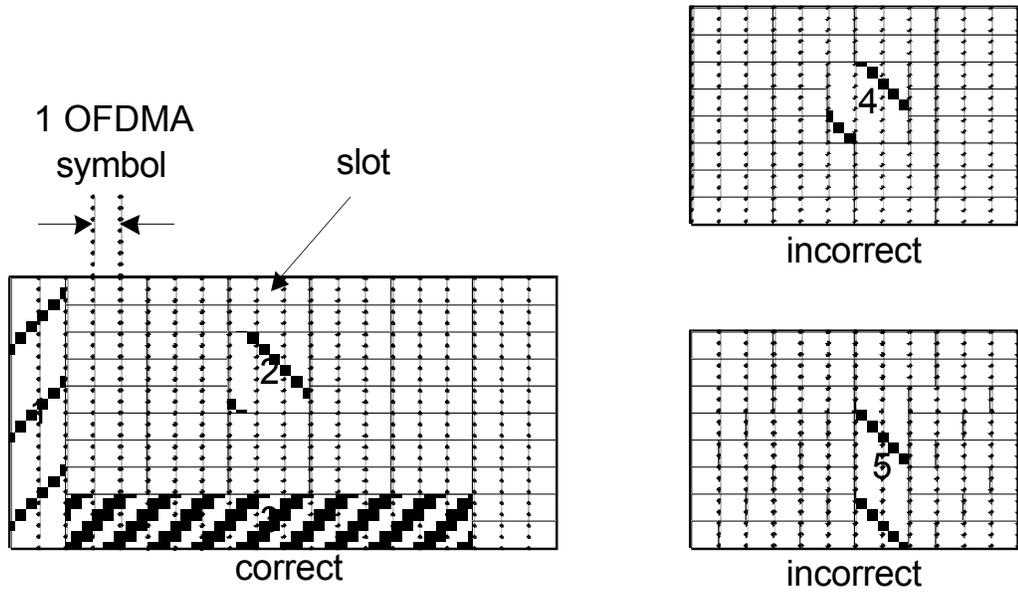
Figure XXX: example of UIUC=12,13 allocation rules.
