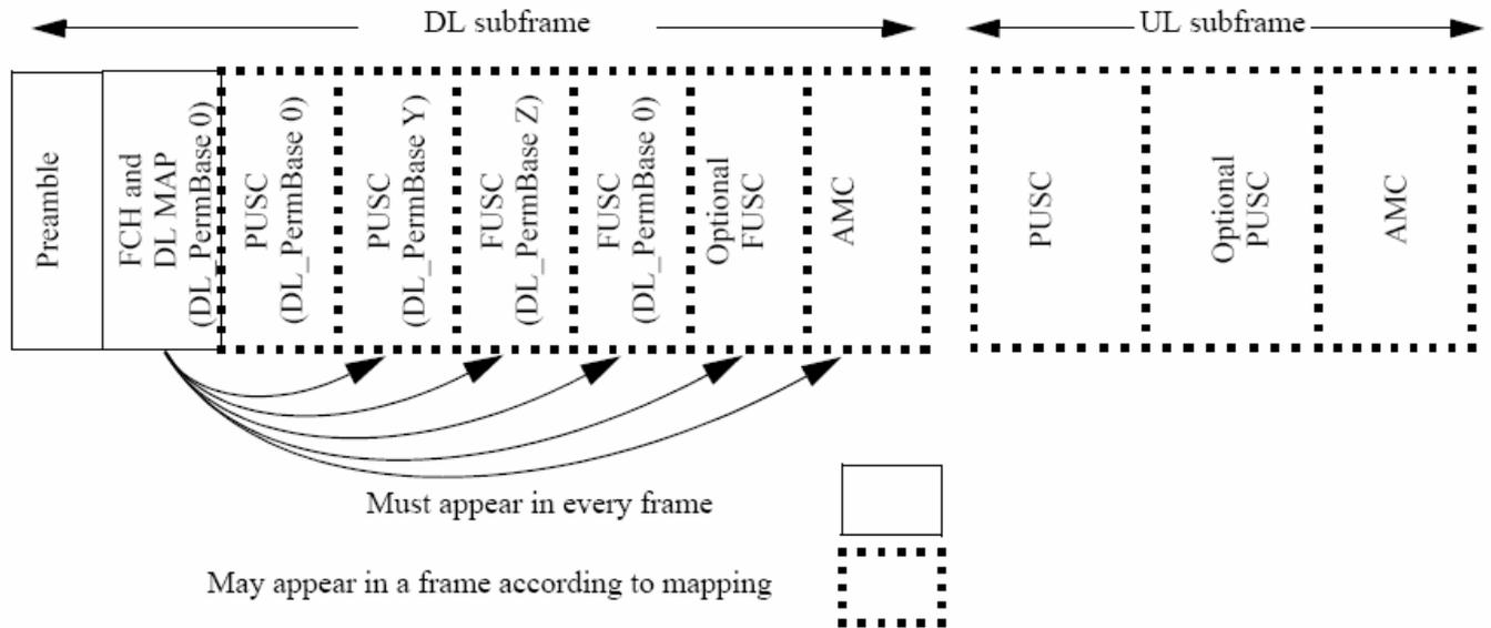
**Figure 219—Illustration of OFDMA frame with multiple zones**
