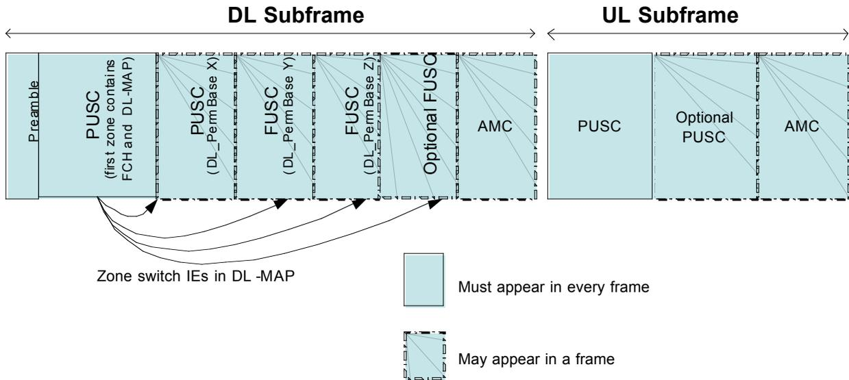
Figure 219-Illustration of OFDMA frame with multiple zones
