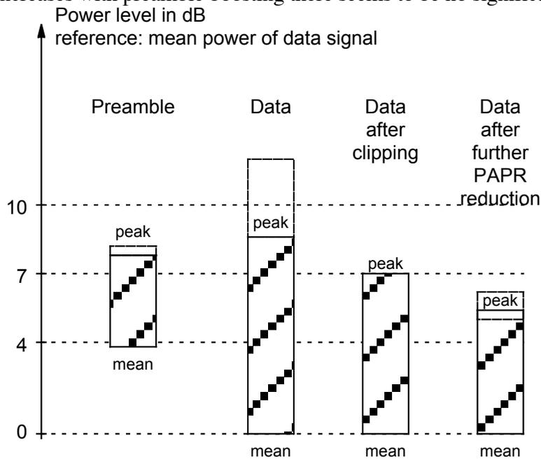
Figure 1: Peak and mean power levels of the preamble and the data signal with and without PAPR reduction
