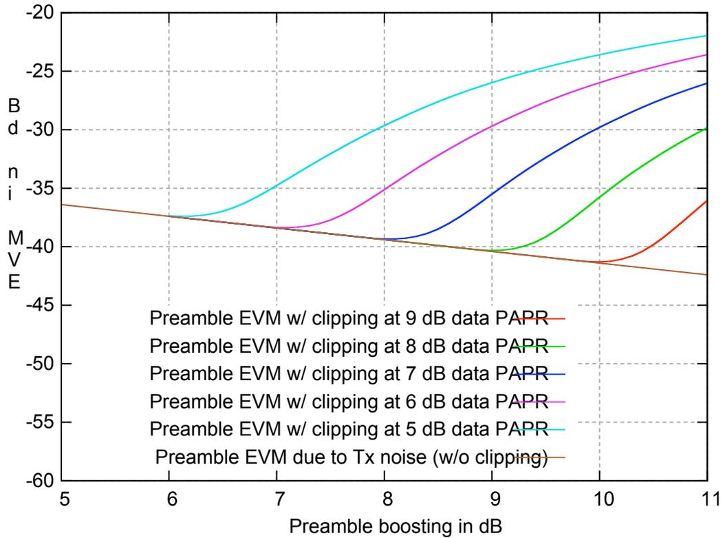
Figure 3: Preamble EVM due to noise and clipping with transmitter noise 31.4 dB below the mean power of the data signal
