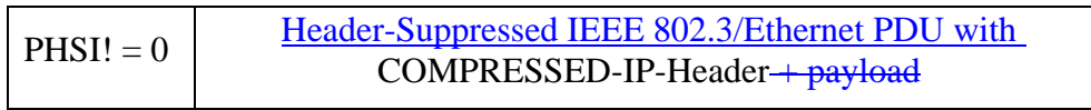
Figure 2022—IEEE 802.3/Ethernet IP CS PDU format, with IP-over-802.3/Ethernet, with both compressed-IP-header and Ethernet header part header suppression
