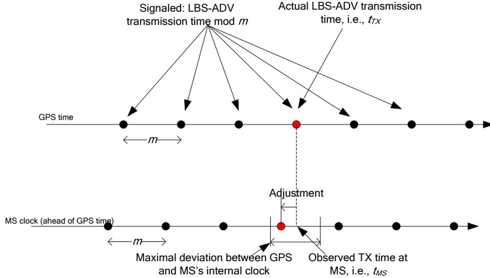
**Figure 3: Adjusting the clock at the MS**
