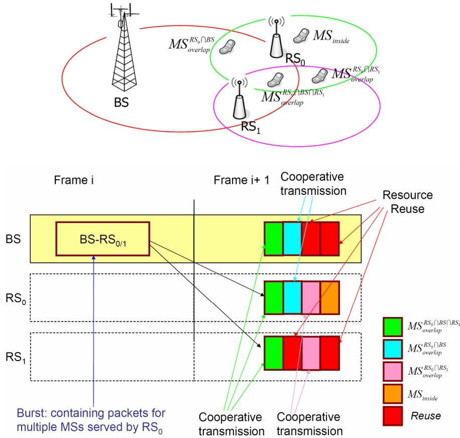
Fig.3 MSs classifications for both diversity gain and resource reuse
