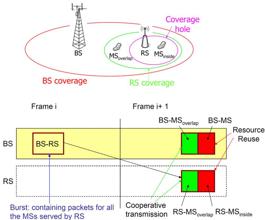
Fig.2 MS classification for both diversity gain and resource reuse in coverage hole application<sup>1</sup>
